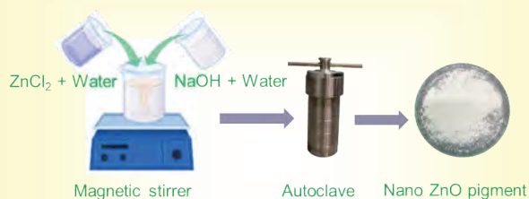
Fig. 1. Fabrication of ZnO nanoparticles by hydrothermal method
