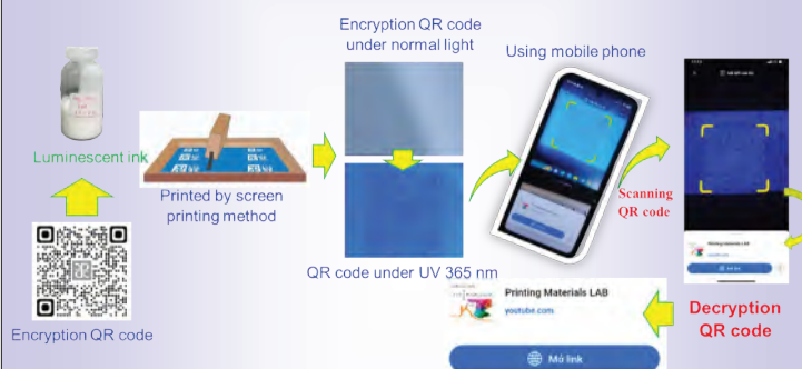
Fig. 6. Applications ZnO nanostructures for security ink
