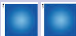
Fig. 8. AM radial gradients (round and ellipse) are smoother than FM radial gradients (20 \mu m and 24 \mu m)
