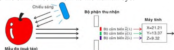
Figure 1. Operating principle of the colorimeter
