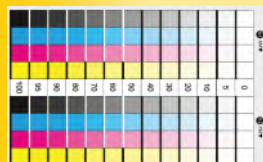
Fig. 4. Dotgain of 50% (AM screening is acceptable; FM screening is higher than the technical guideline value (30-36% vs 28%)
